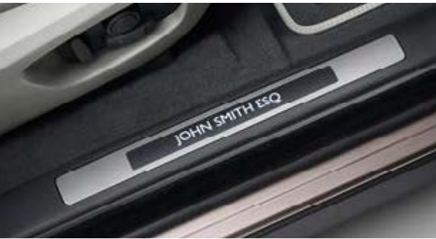
Sill Treadplates – Personalised VPLCS0343PVJ – Ebony VPLCS0343LAA – Lunar (not shown) Personalised illuminated treadplates allow you to choose a personalised message using an approved set of fonts/typefaces which will be highlighted in White illumination when the front doors are open.
