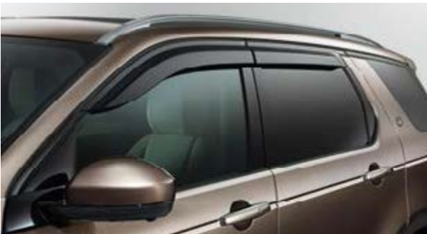
Wind Deflectors – Side Windows VPLCP0258 Wind deflectors for side windows to help to improve comfort levels in the cabin when driving with windows open, by reducing air turbulence and noise and allowing fresh air to be circulated in the cabin.
