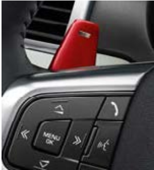
Gearshift Paddles VPLVS0187MMU – Aluminium VPLVS0187CAY – Aluminium Red Complete the look and feel of your steering wheel with premium aluminium paddles. Gearshift paddles are machine polished, anodised and hand brushed to provide exceptional wear resistance with a premium finish.
