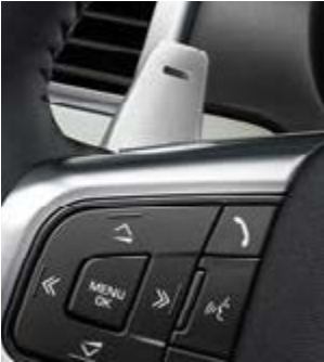
Gearshift Paddles VPLVS0187MMU – Aluminium VPLVS0187CAY – Aluminium Red Complete the look and feel of your steering wheel with premium aluminium paddles. Gearshift paddles are machine polished, anodised and hand brushed to provide exceptional wear resistance with a premium finish.
